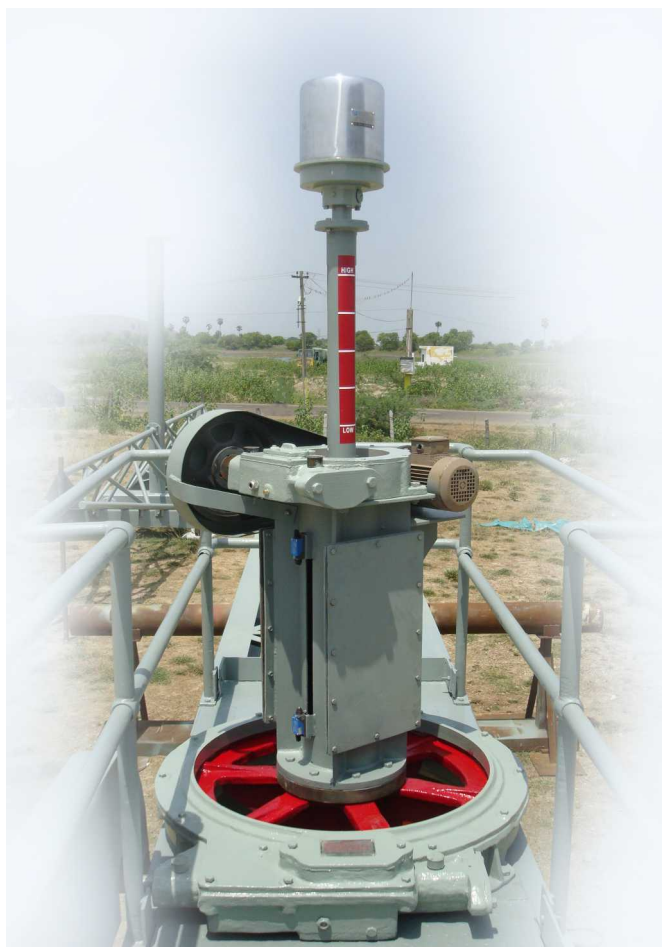
Motorized lifting device with slip ring assembly
